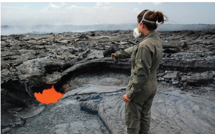
A geologist uses a radar gun to measure how fast the lava is moving during an eruption on the Big Island of Hawaii.
